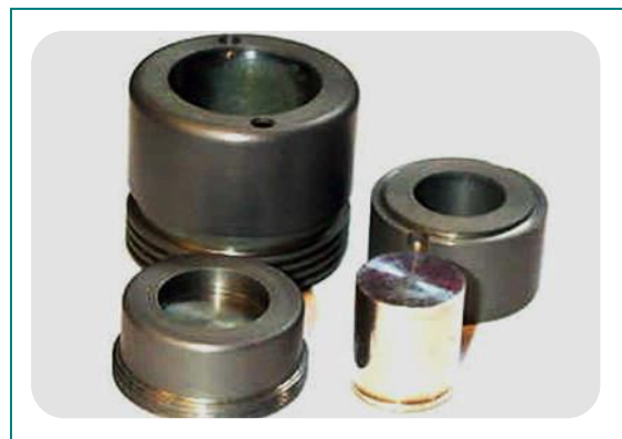
Figure 5: Cs-137 source used for radiotherapy, the same as the one used in Goiania hospital chloride
